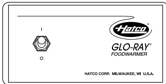
Control Panel w/ I/O (on/off) Toggle Switch.
